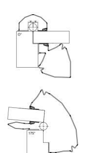
Draw a horizontal line (using a soft pencil) at a distance of 15mm from the bottom edge of the door and at same point on the door frame both on the inside and hinge side (See diagram 1).
