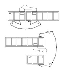
We advise against using screws on metal, aluminium & PVC doors and frames. We therefore recommend using tape. It is often not possible to fit the narrow strip because of a different hinge type, unless the narrow strip and click strip are cut and fitted above and below the unprotected hinge. We strongly advise against this!
