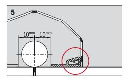
Clicking the narrow strip into the click strip After both narrow and click strip have been correctly fitted, the edge of the narrow strip can be clicked into the click strip starting at the top (See diagram 6).
